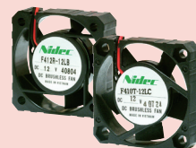
F412R/F410T ●風量: 0.11 m³/min, 0.15 m³/min ●静圧: 15.0 Pa, 26.0 Pa / 10.0 Pa, 23.0 Pa ●騒音: 16 db (A), 23 db (A) / 12 db (A), 18 db (A) ●定格電圧: 5 V, 12 VDC ●□ 41 mm / □ 40 mm
