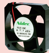
F614T ●風量: 0.36 m³/min ●静圧: 20 Pa ●騒音: 23 db (A) ●定格電圧: 5 V, 12 VDC ●□ 62 mm
