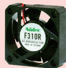
F310R ●風量: 0.09 m³/min, 0.06 m³/min ●静圧: 14.0 Pa, 23.0 Pa ●騒音: 13 db (A), 17 db (A) ●定格電圧: 5 V, 12 VDC ●□ 30 mm
